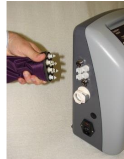
Attaching support cylinder connection plate On Easy Air XL (model 8300)
