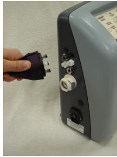
Attaching support cylinder connection plate on Easy Air LR (model 8200)
