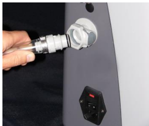
Attaching main air delivery line
