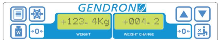
**Zero Weight Change** press and hold to change the displayed weight change to zero.
