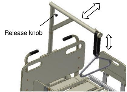
**Warning:** Do not allow the patient to use patient helper unless the boom is locked in the position shown to the right. Failure to do so may result in injury or equipment damage.
