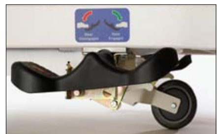
A center-mounted fifth wheel provides an additional pivot point to turn the bed in a tighter arc. The fifth wheel retracts to clear the under-bed space.
